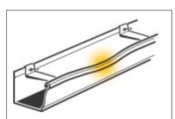
Rain gutters are commonly installed with spaced hangers that cause weak spots on the gutter between each hanger.
